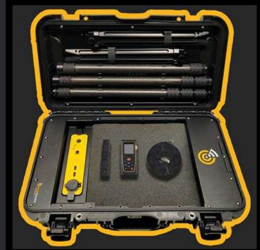
**3.** Remove the stabilizer legs, poles, mounting bracket, ethernet cable and any other tools you'll require for your survey.
