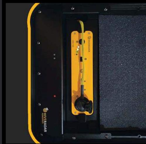
**2.** Power up. Connect the 12 volt plug into the receptacle on the battery. Press and hold the button until the indicator lights come on. Check the small indicator lights on the PowerPack below the battery to ensure that the PoE injector has power.
