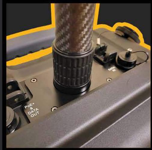
**7.** Connect the remaining poles. Unscrew the cap at the top of the case and screw in the lower pole assembly.
