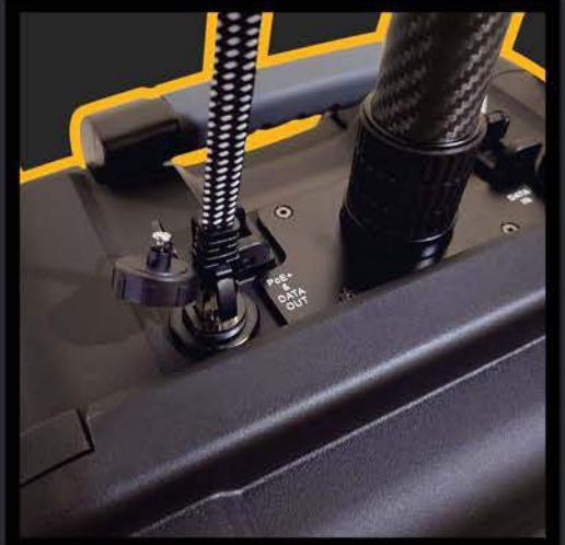
**9.** Connect the other end of your ethernet cable to the ethernet port labeled "PoE+ & data out"
