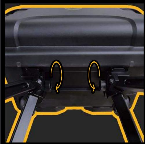
**4.** While the case is still on its back, connect the two stabilizing legs. Loosen the clamp all the way, line up the locking mechanism and tighten. The tightening knobs should be facing inwards. Extend the legs out and stand the case up.
