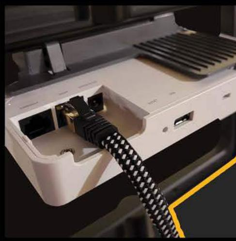
**8.** Connect one end of the ethernet cable to a port on the AP that takes the PoE input.
